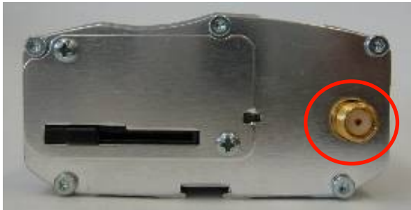
Figure 16. Main RF Connector for the FXT001, FXT002, FXT00, and FXT007
